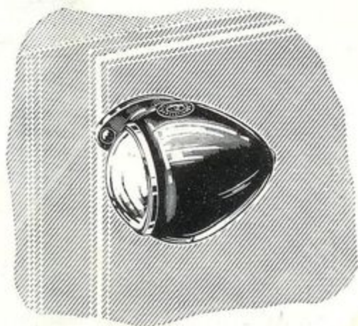
"Concealed Cable" pattern Lamp fixed to sidecar body.
