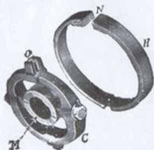
Thrust Lever and Expanding Ring.
