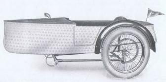
No. 3. Standard Sports, body made of frosted aluminium panels picked out in black. Trimmed in antique red.
