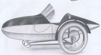
No. 1. Super-Sports, body made of aluminium panels, lower half frosted finish, upper panels black enamel, lined gold. Trimmed in antique red. Supplied complete with screen.
