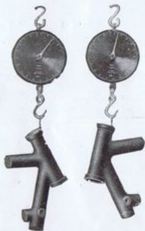
The head lug stamping weighs 9.2 lbs. before machining.
