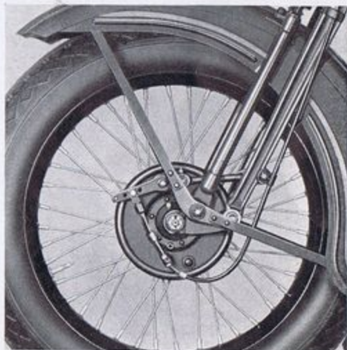
Front brake lining on the new 45 Twin is molded to provide smoother, surer stopping. Molded linings are also used on front and rear wheels of Big Twin.
