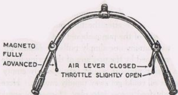
THE CORRECT LEVER POSITIONS FOR STARTING ENGINE WITH OLD PATTERN DOUGLAS CARBURETTOR
