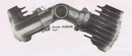
the port. An air-tight joint, which yet allows for cylinder expansion, is in this way obtained.
