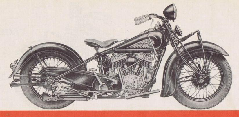
BRAKES—Front and rear wheel brakes, internal expanding.
