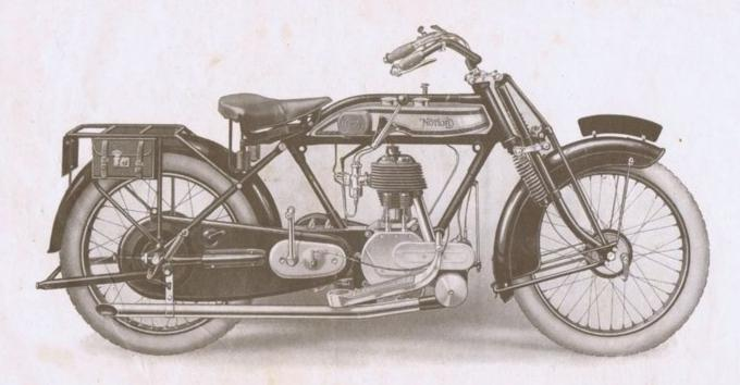
The NORTON "BIG FOUR" Machine here illustrated is identical with the machine described on the previous page, with the exception that a Norton 4-speed Gear Box is fitted and a totally-enclosed Chain Drive. This Box gives the following ratios:—Top. 5.34; Third, 6.95; Second, 9.02; Low, 15.9.
