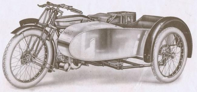
Designed for the use of riders who object to the bulk and weight of the purely Tourist types. This model, the body of which is of Polished Aluminium, is attractive, comfortable and — unlike most of the "Light" types— very well sprung. A removable back seat, adjustable for position, and a well-padded loose Cushion Seat, are standard, whilst the semi-streamline contour of the body reduces wind resistance to a minimum. The Chassis is identical with that of the "Standard" Model.
