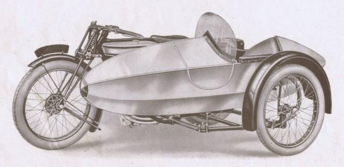
This body has been evolved for the requirements of those who, whilst desiring a light Sidecar of "sporty" appearance, also insist on comfortable and roomy accommodation for the passenger, which is not always found in the orthodox Sporting Sidecar. The body is pleasing in appearance, being made in polished aluminium. The chassis is of the "De Luxe" type.
