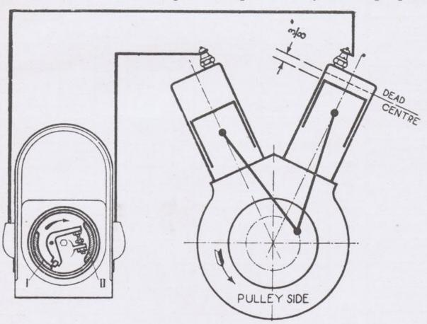
ed by the cam. The cam for the REAR cylinder is marked No. I and is the one following the shorter space between the two cams, when considered in the direction of armature rotation. (See diagram). The magneto sprocket must then be pushed on to the armature spindle, and locked with the nut, care being taken not to move the armature while so doing. The timing should then be verified. In modern magnetos a high standard of reliability has been attained
