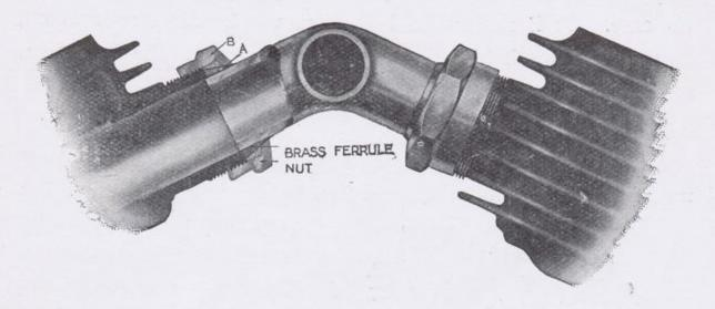
ferrule, and thus tightens it down on to the pipe when screwed to the port. An air-tight joint, which yet allows for cylinder expansion, is in this way obtained.
