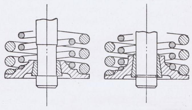
from which they are made is specially selected in our metallurgical department, and is given most careful heat treatment to minimise the risk of breakage. On the O.H.V. engines this risk of breakage is still further lessened by the special fixing for the valve spring.
