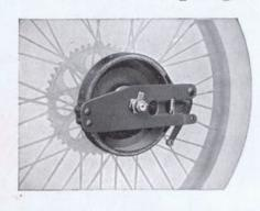
There are no sliding parts to bind. This brake is free when not in use. It does not drag and the rider gets the full power of the motor immediately upon release of the pedal.
