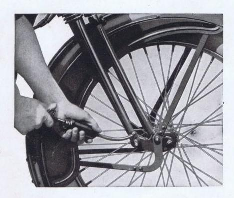
It is only necessary to hook the cap of the Alemite lubricating gun over the fitting and turn the handle. The lubricant is forced right where it is needed under five hundred pounds pressure. A half back turn of the handle releases the pressure and the gun is then slipped off ready for the next fitting. The entire operation takes only a few seconds.
