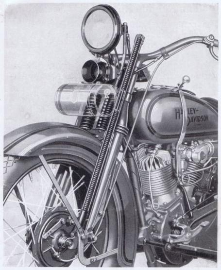
Three springs — main, auxiliary and recoil that go all the way down to the bottom of the frame, float the rider over the bumps and ruts of the road.
