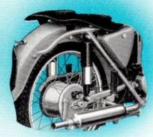
LARGE HUBS The large aluminium alloy Hubs with the very efficient 6in. diameter Brakes fitted to the Special Equipment Sports Model greatly enhance the appearance.
