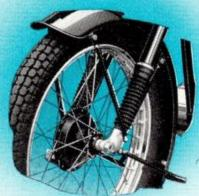
FRONT FORKS **EXCELSIOR Telescopic Forks robustly** constructed provide perfect control and comfort at all times. Phosphor bronze bushed with oil seals and rubber "gaiters" to protect sliding members.
