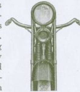
The shock reducing, comfort giving, double spring fork of models 22FD and 22JD
