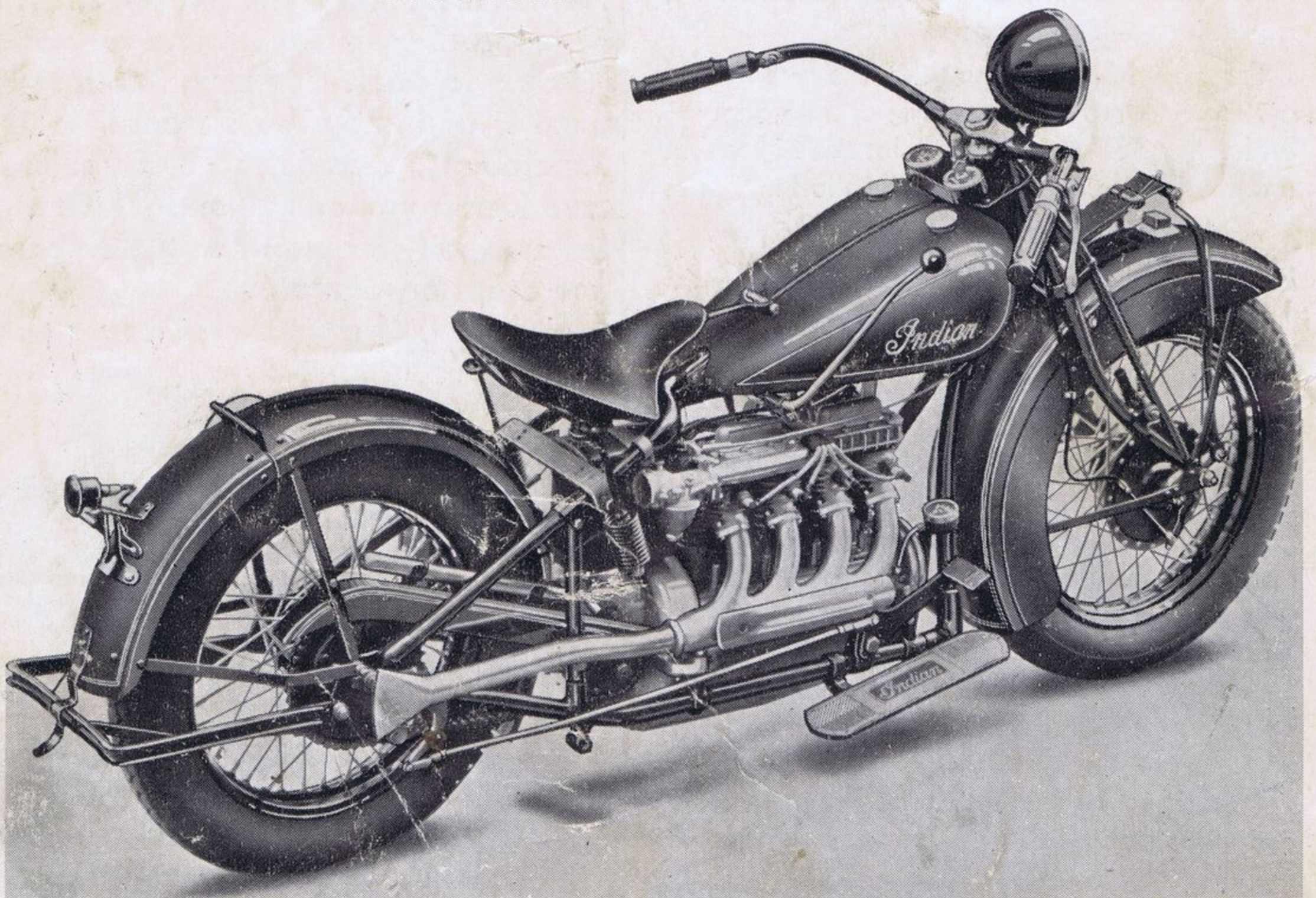
A motorcyclist's view of the new 1932 Indian Four showing the new higher front end, the new wider fork spring, the new front mudguard, new twin steel gasoline tanks, new instrument panel, new footboard position, new saddle position, new exhaust tube and other features which all go to make up the finest motorcycle built in America.
