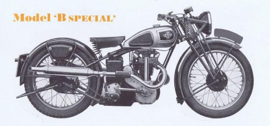
ENGINE . Bore: 67 m.m., Stroke: 70 m.m., 247 c.c., Two-port with entirely enclosed Valve Gear, Valves and Springs. Compression—Standard: 7.2 to 1. High: 8.3 to 1, for racing with 50-50 petrol-benzol fuel, optional.
