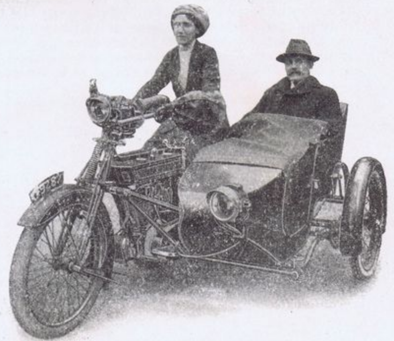
MRS. M. RILEY , of Birmingham—one of the foremost lady riders of to-day—and her 6 h.p. Royal Enfield Side-car Combination.
