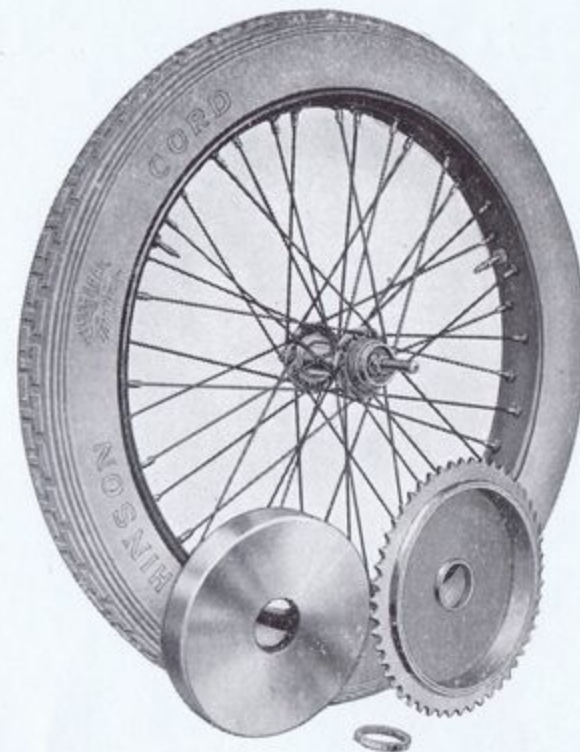
Wheels and Brake Drums are quickly detachable on the new Douglas Models.
