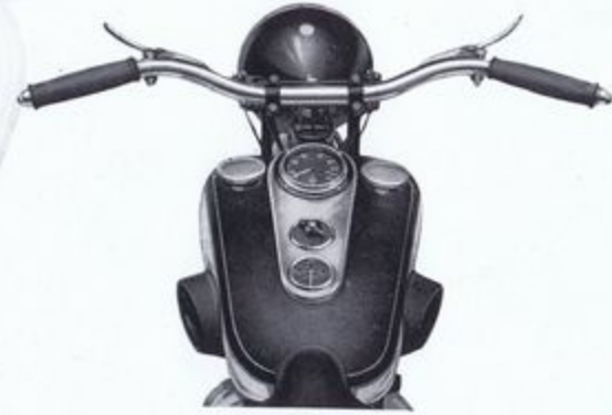
The illustration above shows the arrangement of the Instrument Panel on the Sports Model MG.-31. The Speedometer and Ammeter are lighted for night riding.
