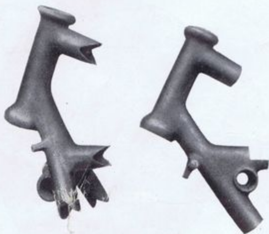
This is the B.S.A. duplex cradle frame fitted to the five models with inclined engines.
