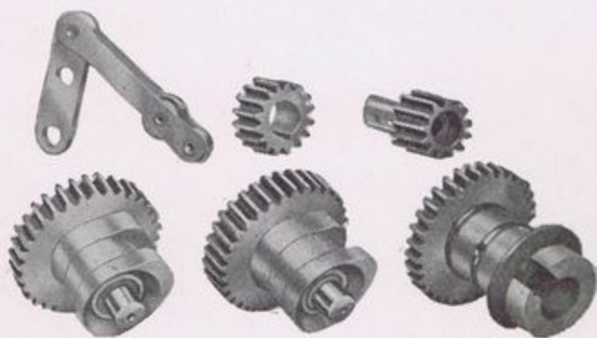
FIG. 25.—THE CAMS AND TIMING GEAR USED ON THE 500 C.C. AND 600 C.C. S.V. ENGINES
