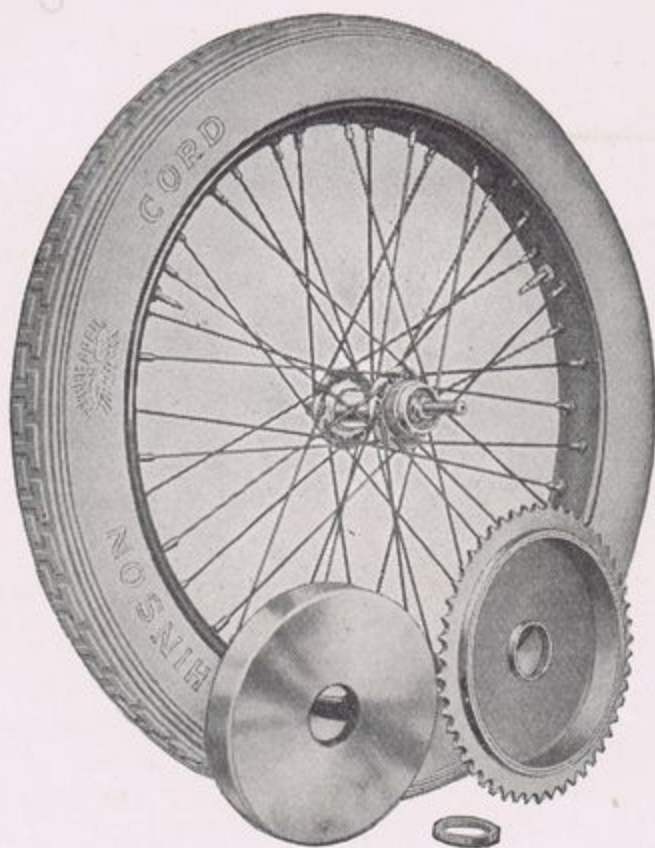
FIG. 19.—WHEEL SHOWING DETACHABLE BRAKE DRUM
