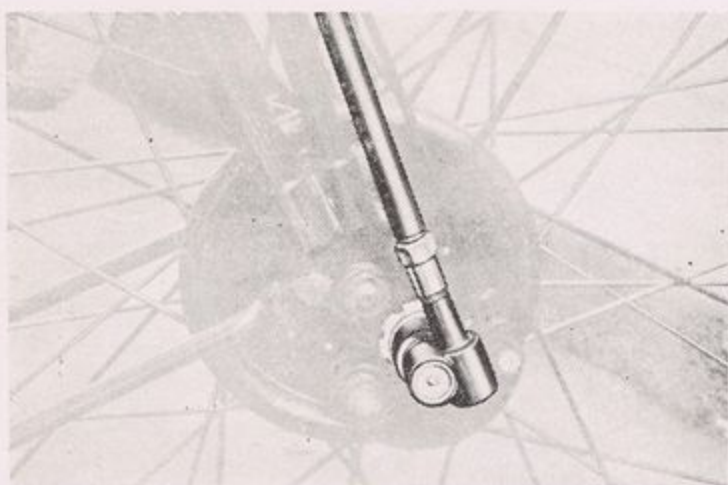
FIG. 6A. THE ENCLOSED FRONT HUB DRIVE FOR THE SMITH SPEEDOMETER
