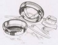
The new B.S.A. filler cap with special cam-locking action, combining quick release with freedom from petrol leakage.
