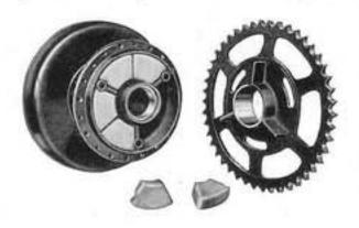
the harshness otherwise present in a chain drive. Both driving and rebound shocks are absorbed by blocks of solid rubber enclosed in the rear driving sprocket.
