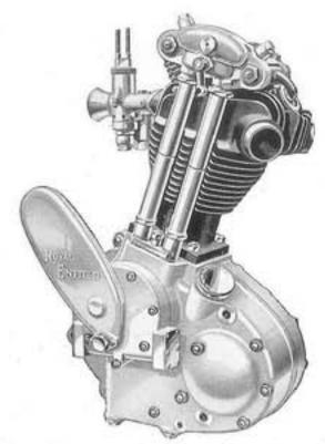
O.H.V. engine) shows the clean exterior of these dry-sump lubricated engines, the system being self contained and without a single external oil pipe, tap, regulator, or other excrescence.
