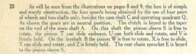
To obtain first gear, the pinions U and X slide to the right until the dogteeth on X engage with those on W, thus in effect clutching W on to the layshaft B, so that the drive is taken from A through V and W to B, and then through Z and S to the sprocket E.
