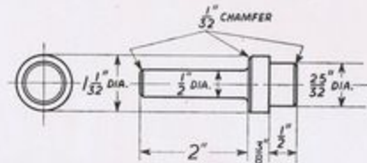
DRIFT FOR REMOVING GEARBOX MAIN BALL BEARING.
